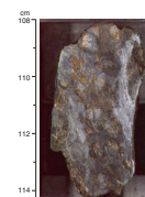
F43. Clay and iron oxyhydroxide weathering of harzburgite, p. 95.
