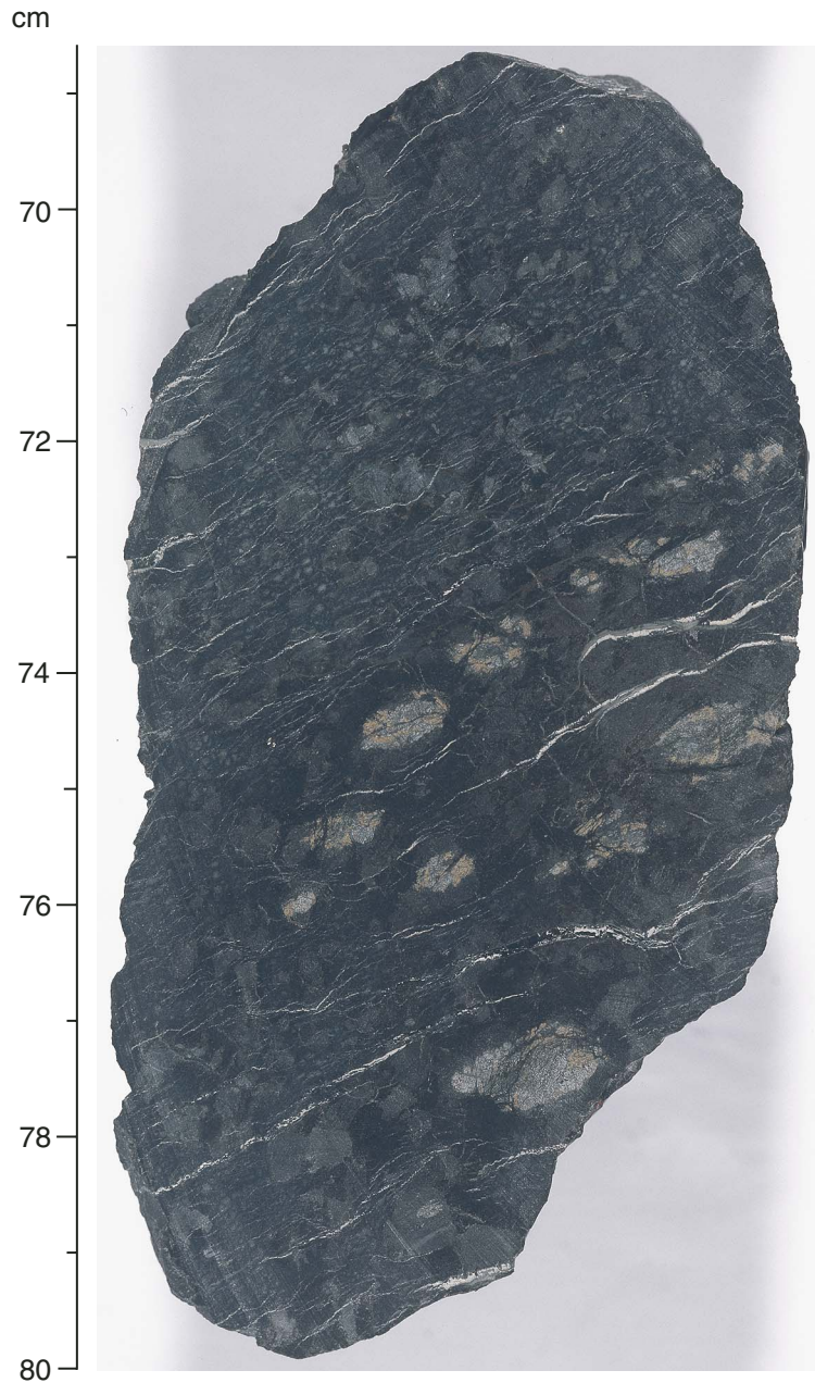
Figure F18. Close-up view of variation of altered orthopyroxene porphyroclasts (in light gray) in an altered harzburgite. Note that modal orthopyroxene is highest between 73 and 76 cm (interval 209-1270C-1R-1 [Piece 11, 69–81 cm]). Figure F17, p. 68, shows an image from a thin section at 72–75 cm.
