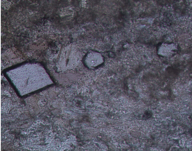
Figure F26. Photomicrographs showing zircon crystals in amphibole layer (Sample 209-1270D-4R-1 [Piece 7, 33–37 cm]) (field of view = 0.7 mm). A. Plane-polarized light: blue filter; image 1270D_002. B. Cross-polarized light: blue filter; image 1270D_003.
