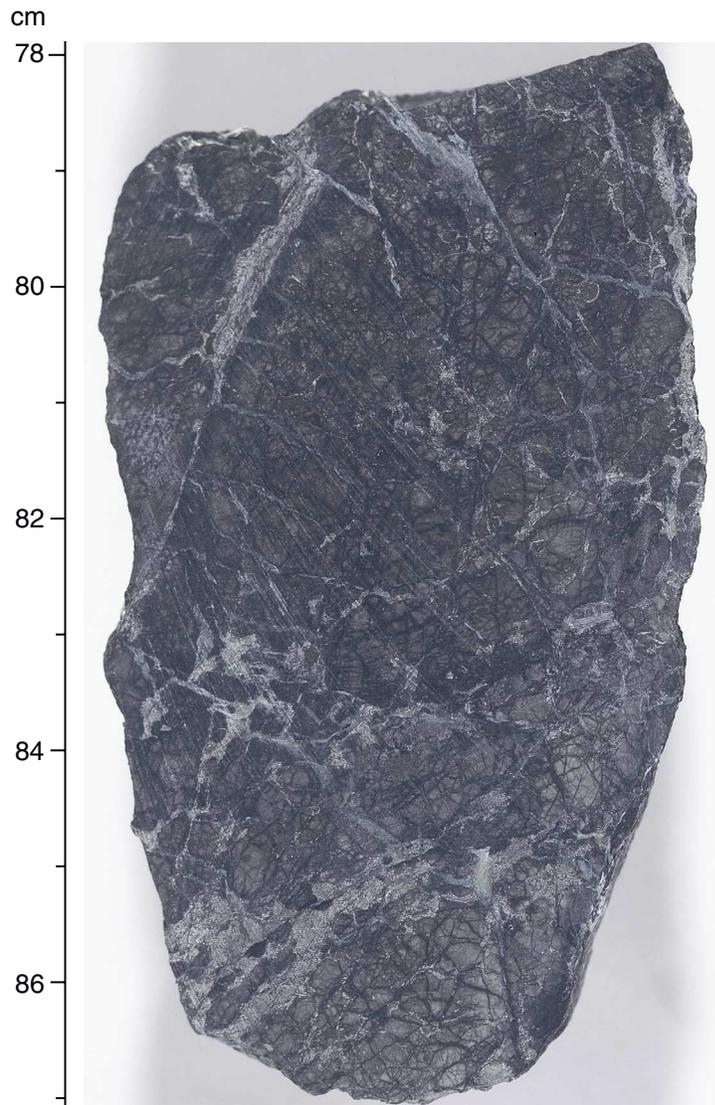
**Figure F10.** Close-up photograph of chromitite pod in dunite. The matrix surrounding chromite in the chromitite pod consists of chlorite (possibly replacing plagioclase) and amphibole. The host dunite intruded by the chromitite is also rich in chromian spinel (interval 209-1271A-4R-2 [Piece 2, 38–48 cm]).
