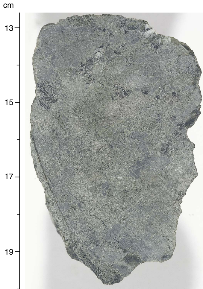
Figure F8. Close-up photograph of altered gabbro (interval 209-1274A-21R-1 [Piece 5, 13–20 cm]).
