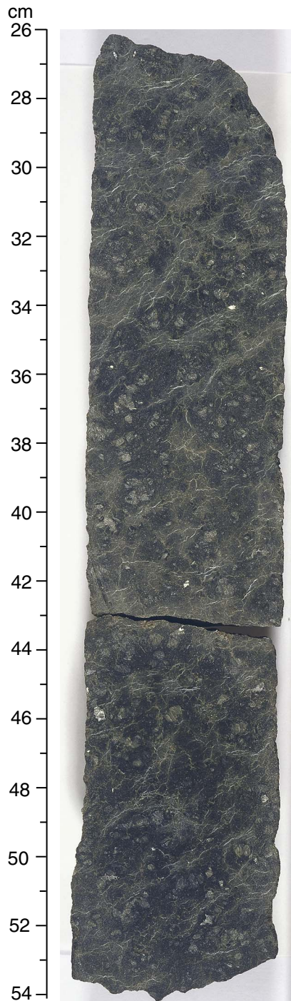
Figure F4. Close-up photograph of typical harzburgite (interval 209-1274A-3R-1, 26–54 cm).
