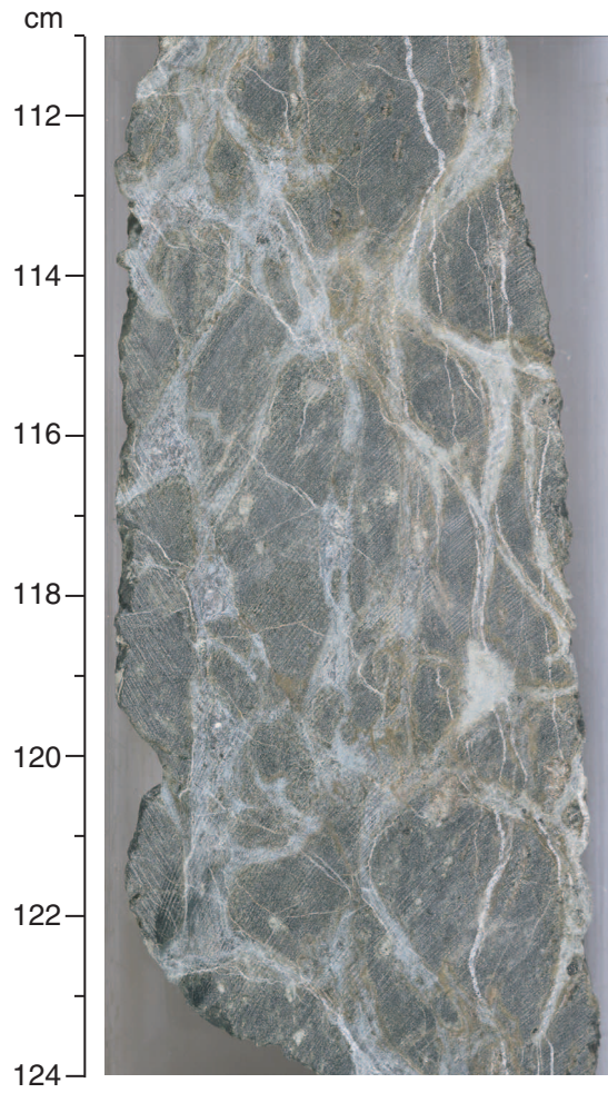
Figure F11. Foliated serpentized peridotite (dark) cut by a network of anastomosing paler greenish veins consisting of calcite and talc (interval 210-1277A-7R-2, 111–124 cm).
