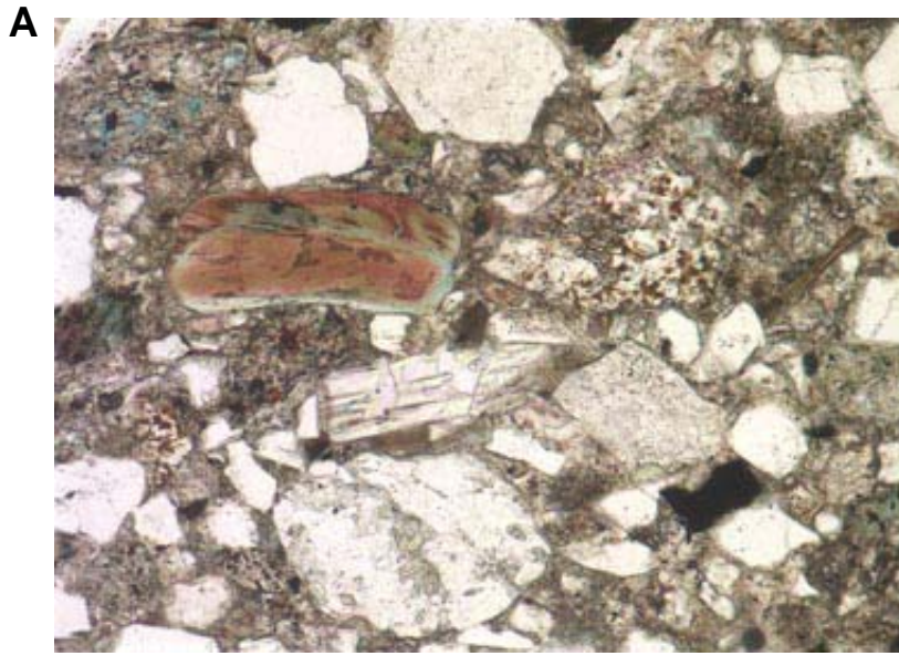
Figure F7. Metasedimentary rock fragments, altered biotite, muscovite/quartz intergrowth, and monocry- stalline quartz set in a microcrystalline carbonate cement (Sample 210-1276A-81R-3, 134 cm). A. Plane- polarized light. B. Cross-polarized light.
