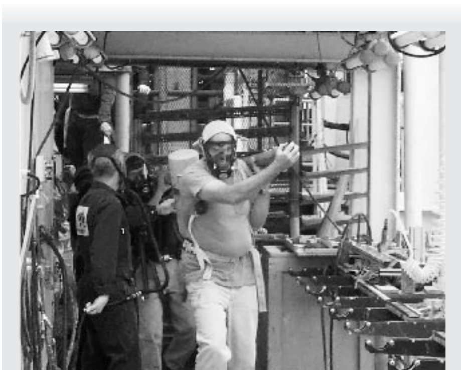
FIGURE 3 Recovering core on the rig floor and cutting/splitting core on the catwalk were difficult because of the high concentrations of poisonous hydrogen sulphide gas.
