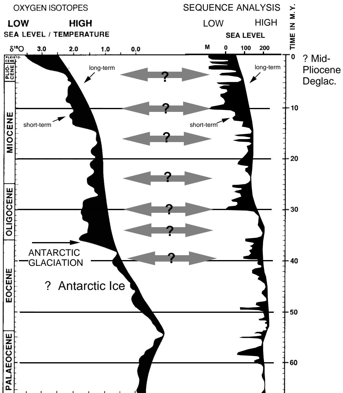
1‰  $\delta^{18}\text{O} = 110 \text{ m sea level or } 4^\circ\text{C water temp.}$
