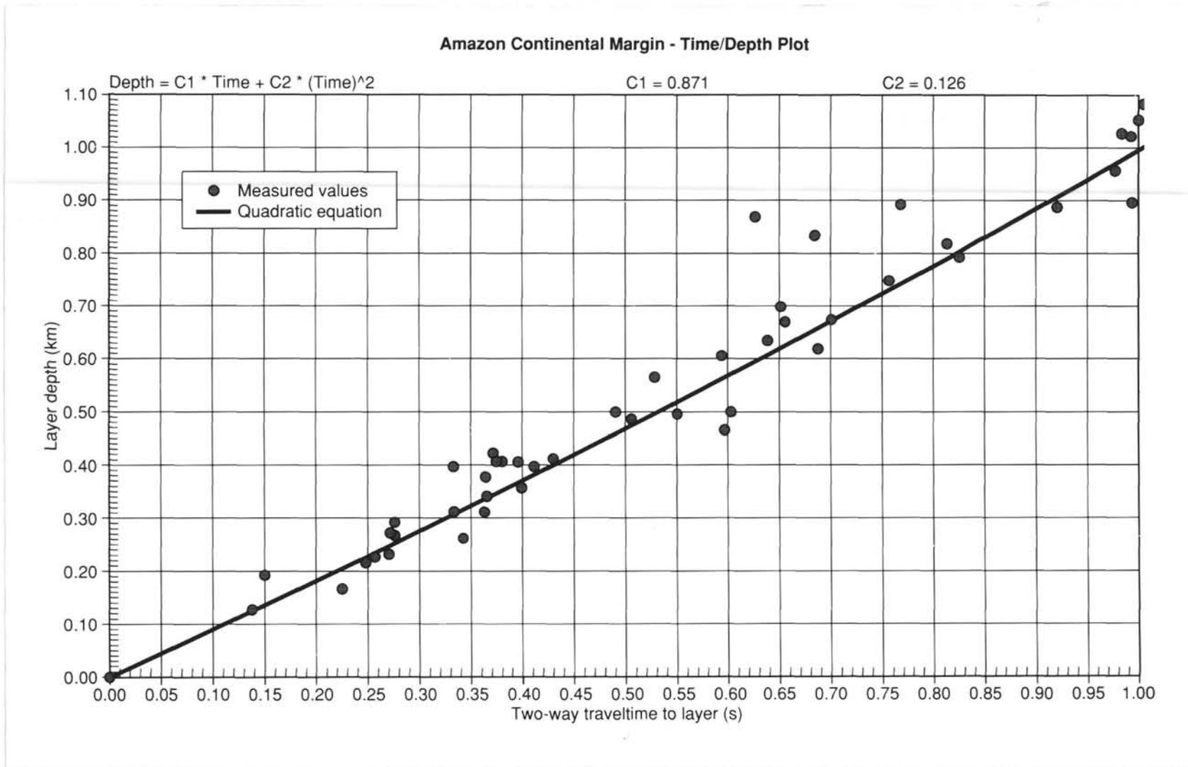
Figure 11. Time-depth plot from sonobuoy data on the Amazon Fan. Some local variation from this plot is expected depending on the sediments at each particular site.
