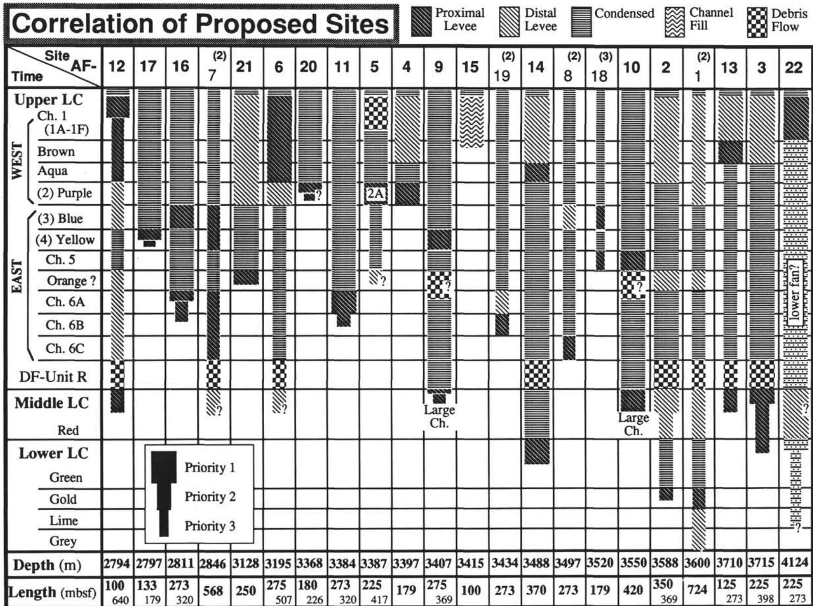
Figure 10. Schematic illustration of the overall relationship between proposed drill sites and the acoustic stratigraphy of the Amazon Fan. Seismic profiles at sites show more precisely the relationships observed. Sites arranged in order of increasing water depth.
