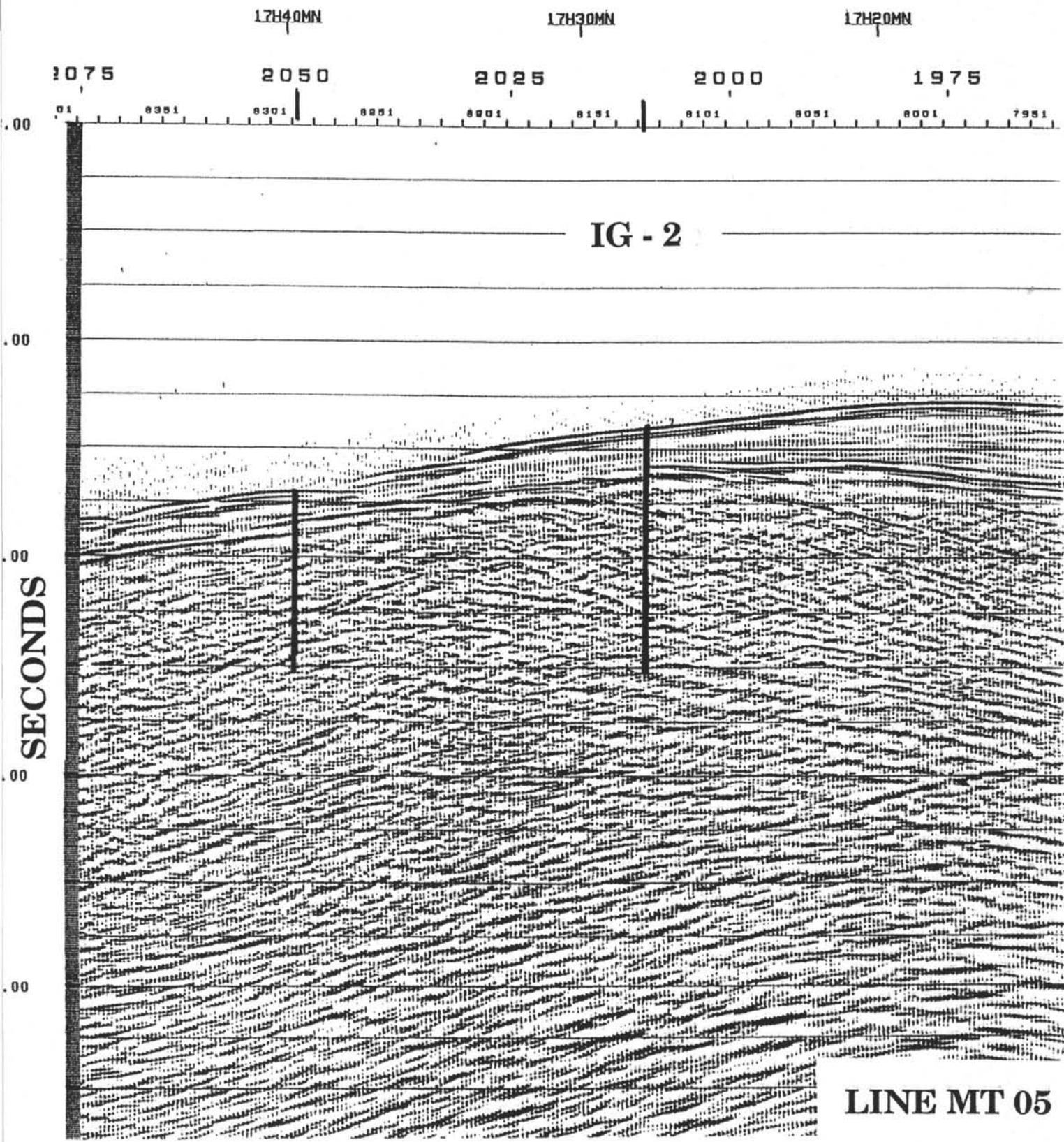
Figure 13. Enlarged section of MCS line MT05 and location of proposed site IG-2.
