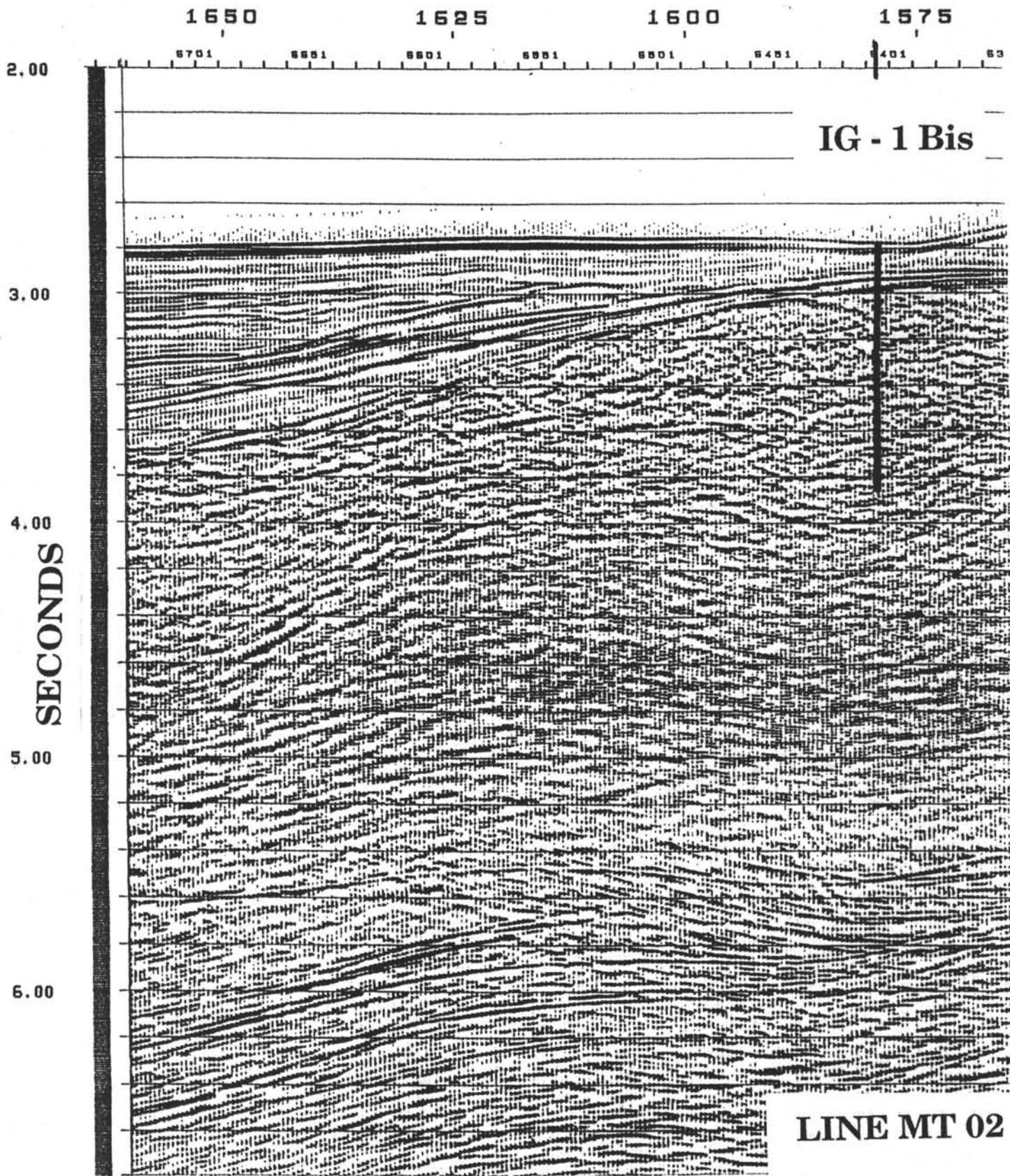
Figure 15. Enlarged section of MCS line MT02 and location of alternate site IG-1Bis
