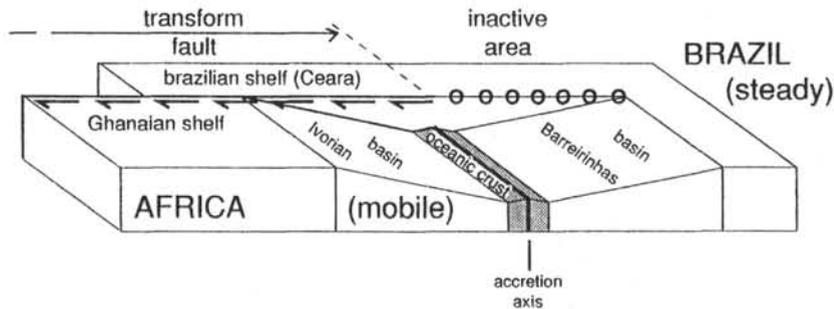
**Figure 10.** Kinematic evolution of the CIG Transform Margin and divergent deep Côte d'Ivoire Basin (view from the north). Brazil is supposed to be fixed. Arrows indicate horizontal and vertical relative motions (strike-slip and dip-slip faults, respectively) between the steady plate and the moving plate.
