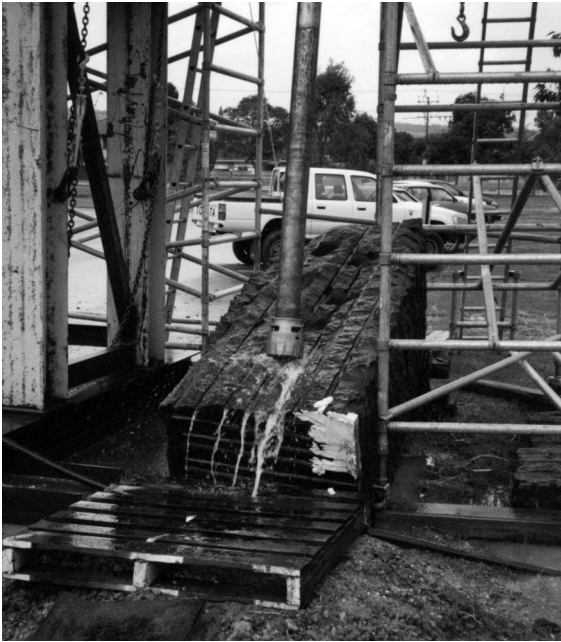
Inclined spudding tests with ring style bit.
