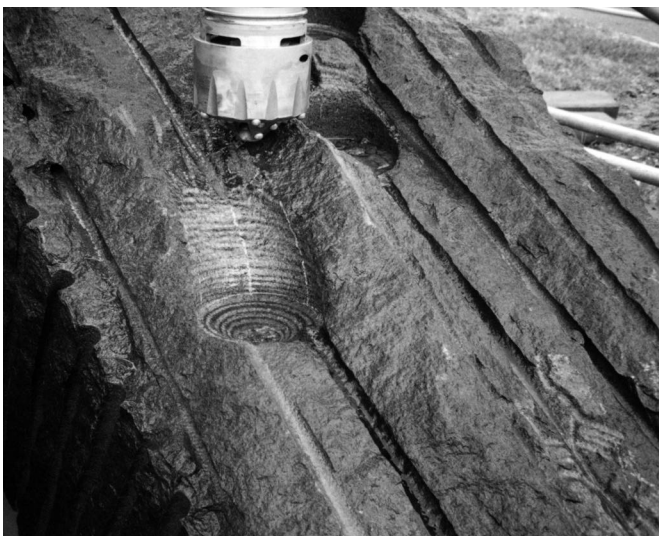
Results of inclined spudding tests. Note: bit walking until securing a toe hold to make hole.
