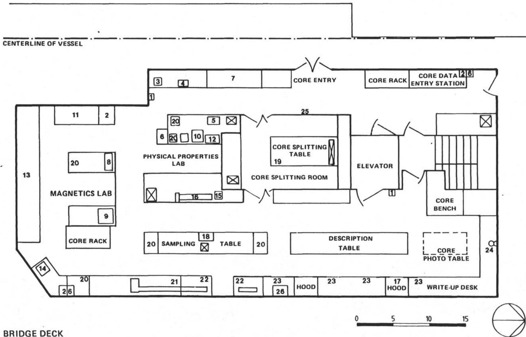
sections are cut longitudinally into work and archive halves in the core splitting room and carried into the sampling and sedimentology labs for core description and sampling.
