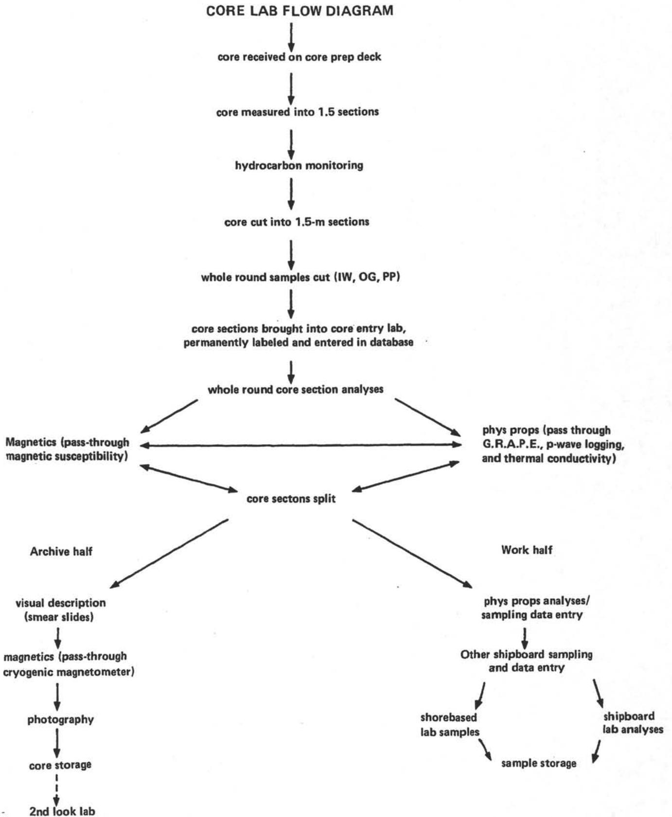
Figure 9. Core lab flow diagram.
