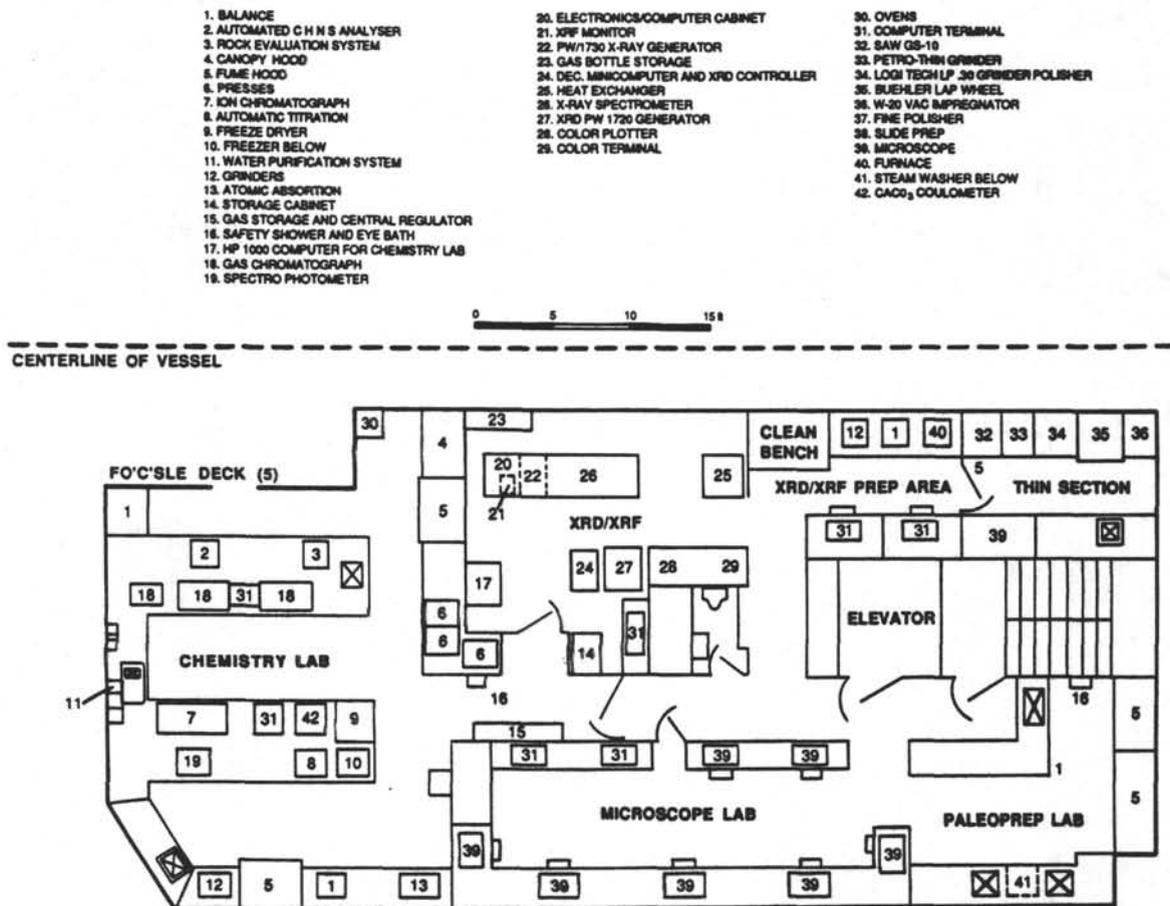
Figure 8. Layout of laboratory stack's fo'c'sle deck, including paleontology preparation (paleo-prep) lab and microscope lab.
