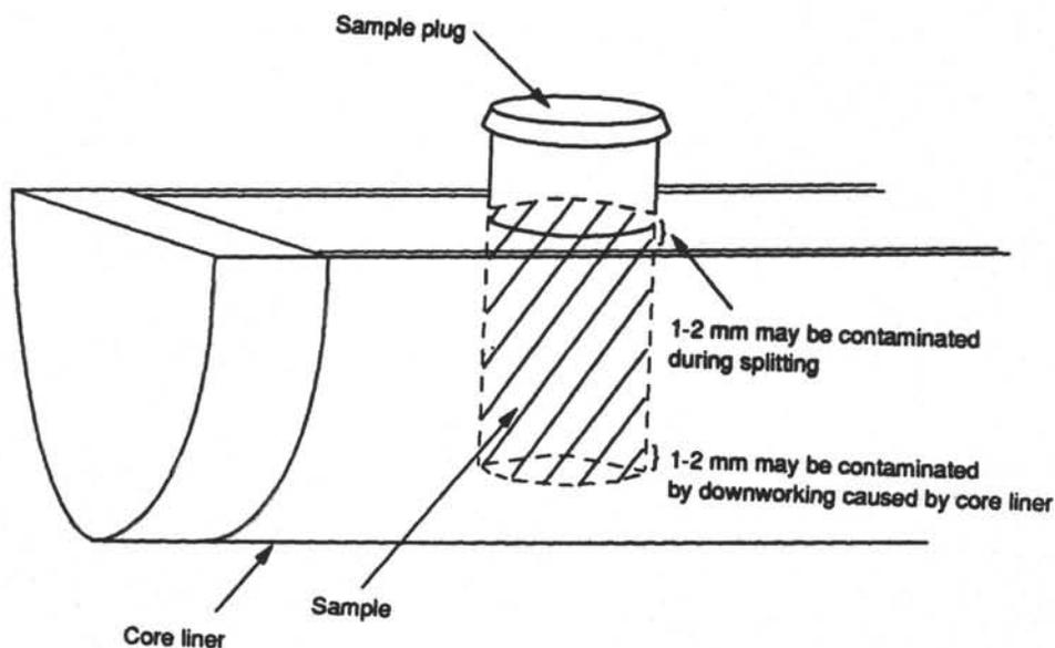
Figure 2. Drawing of a sample plug showing regions of highest potential contamination.
