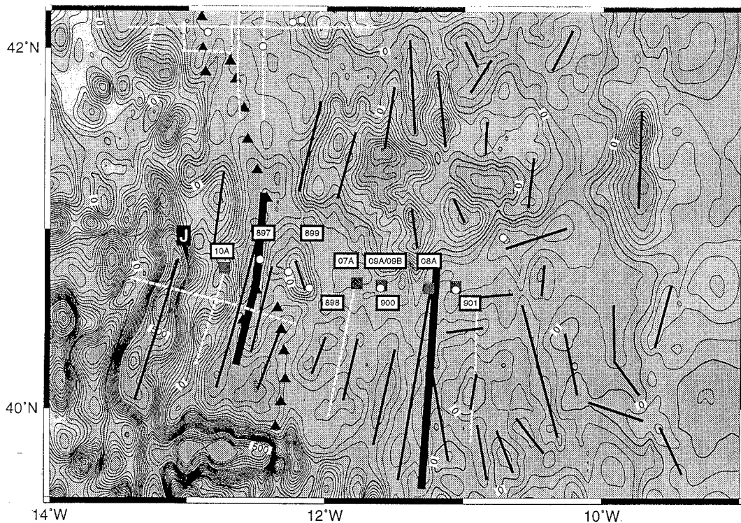
Figure 3. Part of a new reduced-to-the-pole magnetic anomaly chart of the whole west Iberia margin produced in collaboration with the Atlantic Geoscience Centre, Dartmouth, Nova Scotia, Canada (Miles et al., in press). The chart was made from a 5-km gridded data set and is contoured at 25 nT. The main chart is based on over 400,000 sea-surface observations which were corrected to remove the effects of secular variation, high geomagnetic activity, spurious tracks, and systematic cross-over errors. Greater confidence in the quality of the resulting data set allowed the use of the small contour interval. ODP Leg 149 drilled to basement in this area (white dots); proposed sites are shown by squares. The data were reduced to the pole to clarify many features. Major linear trends in the anomalies are picked out by bold lines. The chart clearly shows the strong positive J anomaly which appears just west of 13°W and south of 41°30'N. Between anomaly J and the continental shelf (~9°15'W) other less strong positive anomalies are associated with the shallow region south of Galicia Bank. South of ~41°N the chart can be divided into three distinct zones (bounded by the two broad N-S black bands) based on the character of the anomalies.
