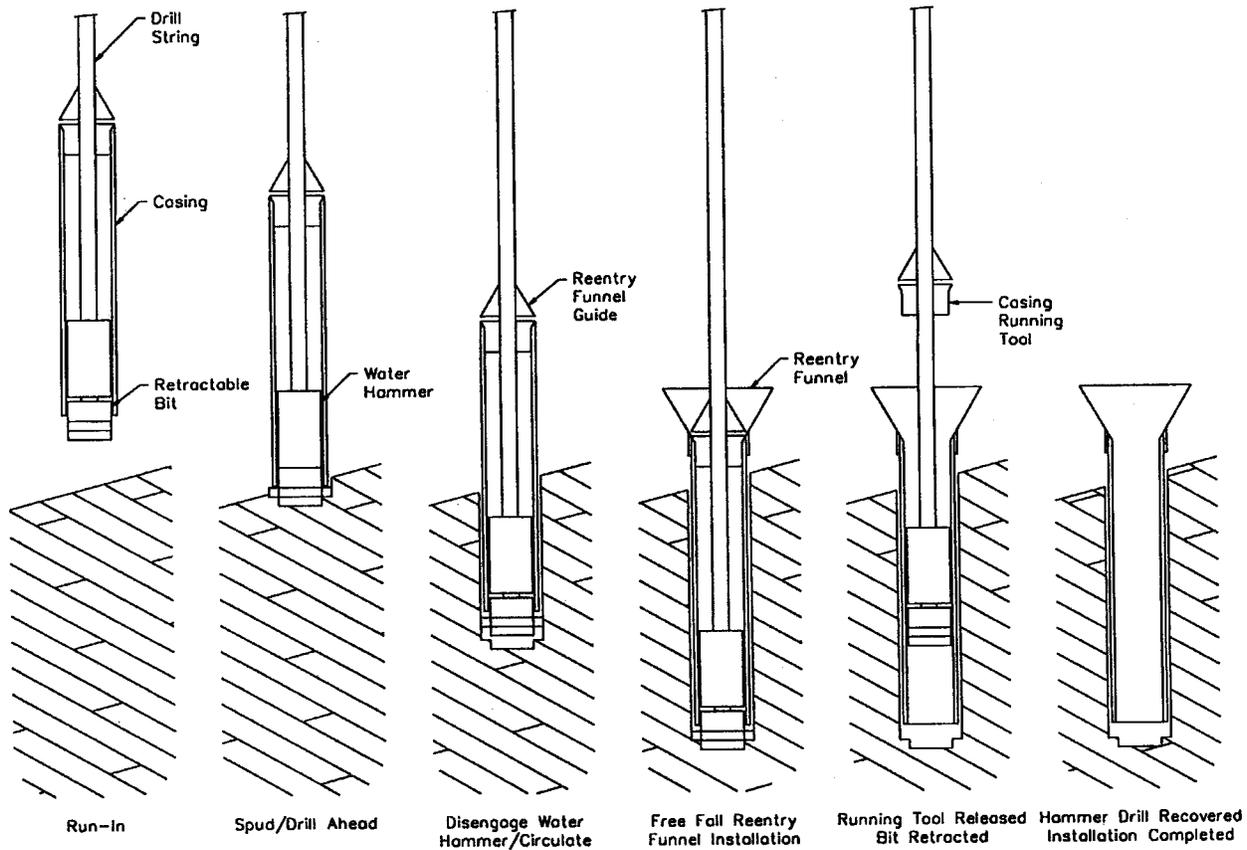
**Figure 2.** Schematic diagram of Water Hammer Drill-In Casing System deployment.
