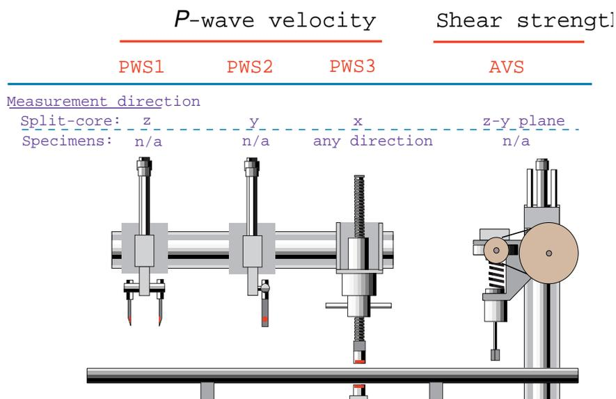
Figure 1—2 Schematic view of the semiautomated instrumentation on the working-half core track. n/a = not applicable.
