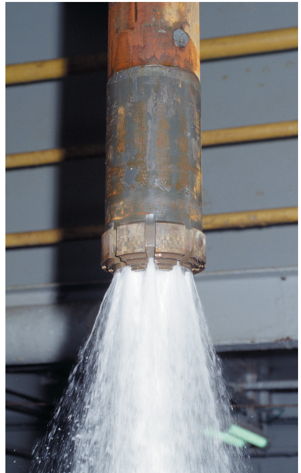
ADCB bit showing circulation test.
