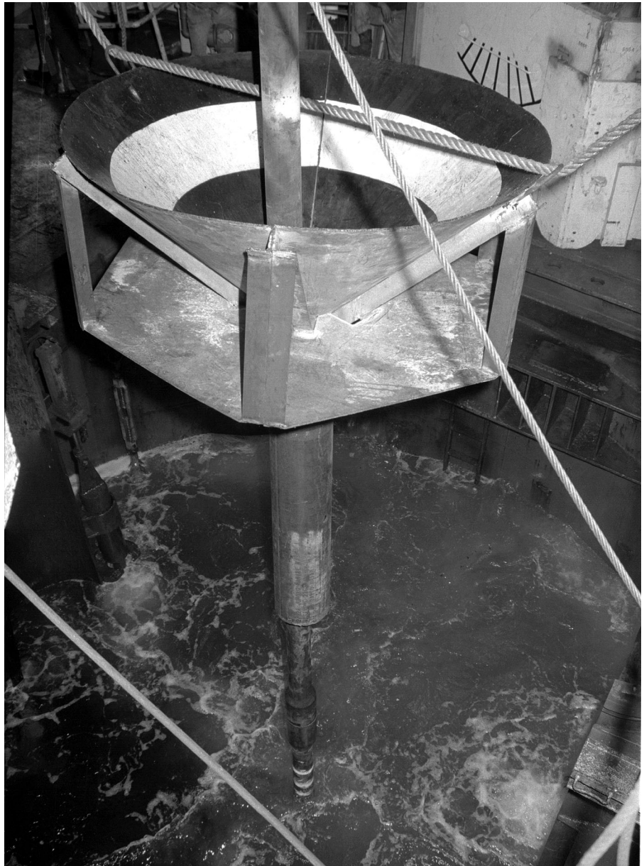
FFF with a 9 ft casing stub installed over the drill string and ready to drop in the moonpool.
