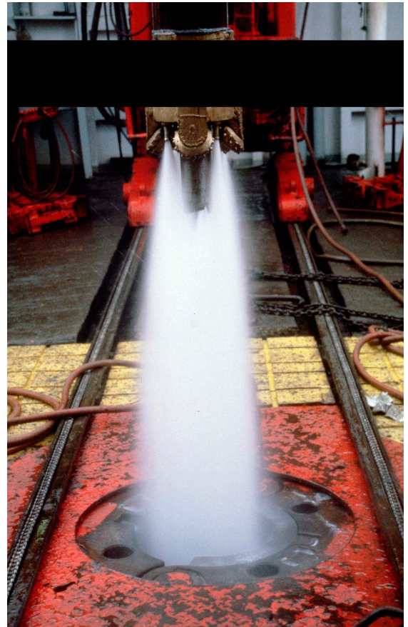
Rig floor flow test of the MDCB.
