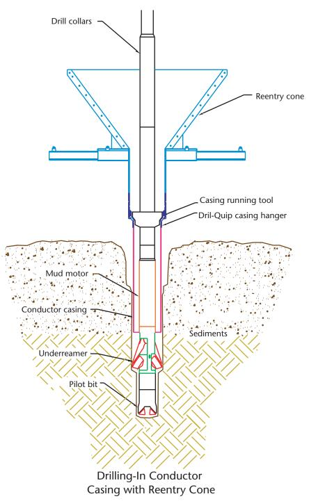
Figure 4. Underreaming ahead of conductor casing in unstable sediment cover to set reentry cone.
