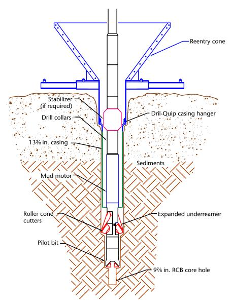
Figure 3. Underreaming (enlarging) 9<sup>7</sup>/<sub>8</sub> in. core hole with an expanded underreamer below conductor casing before running next casing. If a bicenter reamer was used, it would be in the same position below the mud motor as the underreamer.
