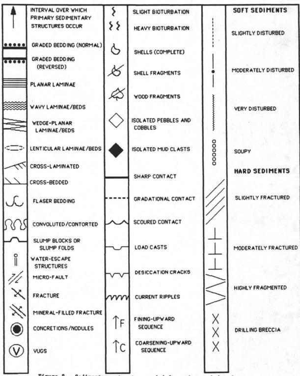
Figure 8. Sedimentary structure and deformation symbol codes.
