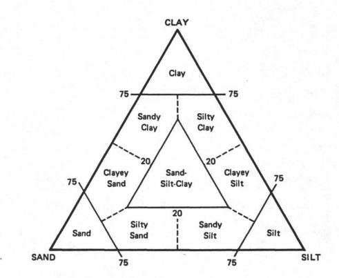
Figure 2. Ternary diagram showing principal names for siliciclastic sediments (from Shepard, 1954).
