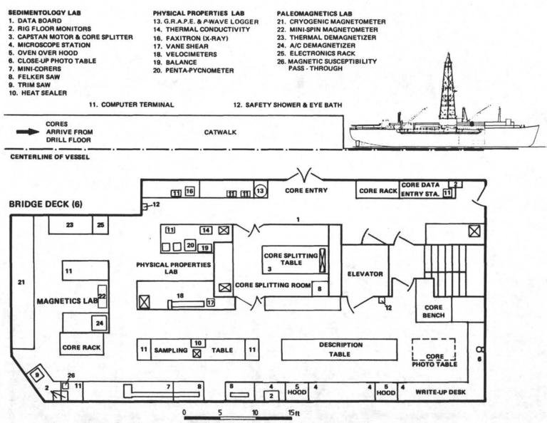
Figure 2. Diagram of the lab stack's bridge deck, containing core entry, core splitting, sedimentology, physical properties, and paleomagnetics laboratories.
