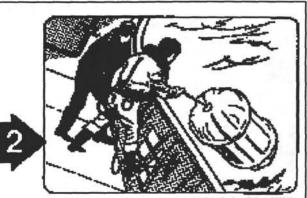
LAUNCHING THE RAFT OVER-BOARD. THE PAINTER HAS, IF NECESSARY, BEEN MADE FAST TO A NEW STRONGPOINT BEFORE LAUNCHING. CONTAINER WILL FLOAT.
